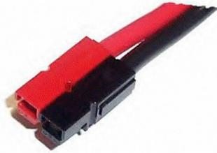
Put the connector housings together before inserting the connector pins in, this is easier when using heavy paired wire.
