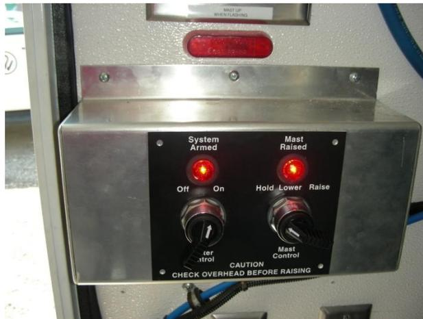
Compressor Arming and Mast Raise/Lower/Hold Switches
